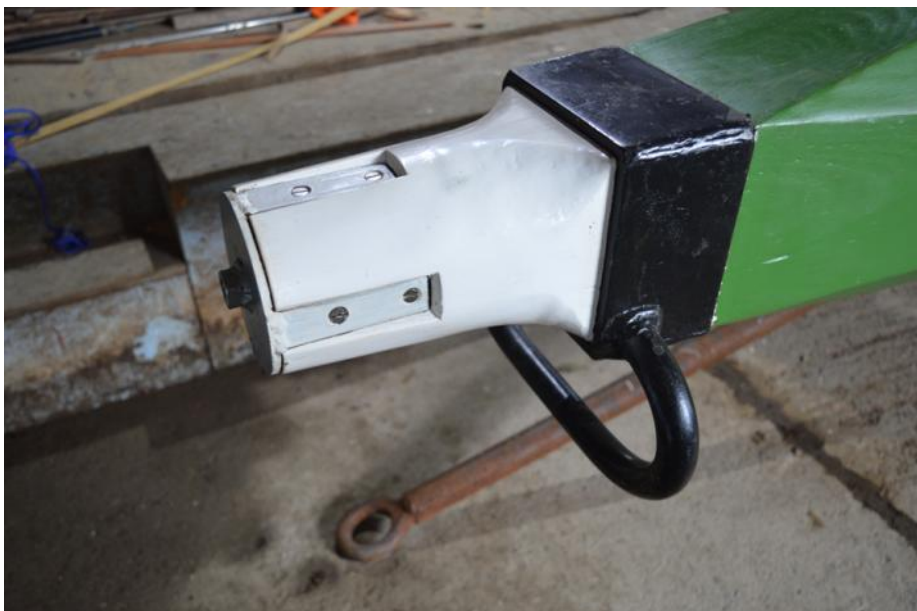
New crane iron at the top of the mast photo: Nigel Gutteridge on 15 September
