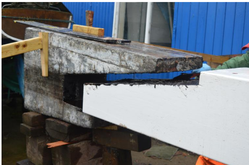
Fitting the mast counterbalance weight on the bottom of the mast Photo by Nigel Gutteridge on 17 September
